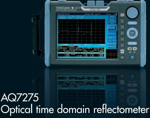
The AQ7275 offers the industry's best performance in terms of event separation capability and the shortest dead zone, less than 80cm, to enable multiple-event detection even when events are close to one another. Its high-speed operation optimises work efficiency, while automatic test functions enable installers to execute tests easily and reliably.
