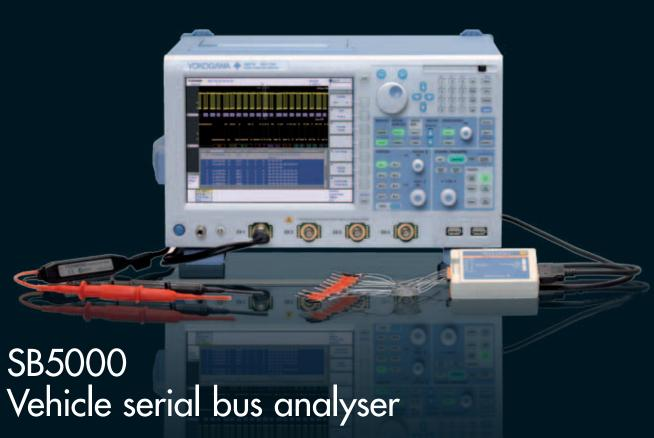
The SB5000 is a serial bus analyser focused on in-vehicle serial bus protocols including FlexRay, CAN and LIN as well as providing UART,  $\rm l^2C$  and SPI trigger and analysis capabilities. It performs FlexRay signal integrity testing (SI Voting), eye-diagram analysis and bus driver electrical parameter measurement, and provides simultaneous analysis of analogue and logic channels, and simultaneous observation of any two serial buses.
